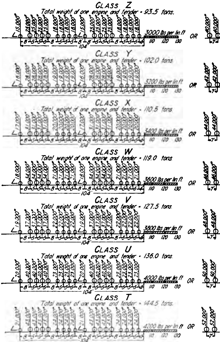
Fig. 6a. The Compromise Standard System of Live Loads for Railway Bridges.
